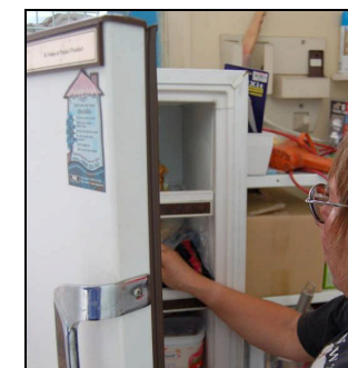
Check the air-seals on your fridge door - replace if perished and leaking air
